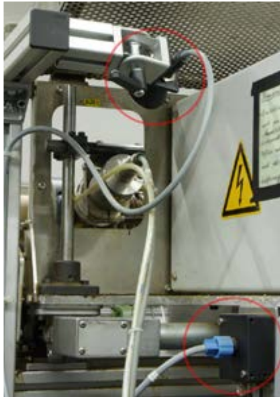
Fig. 6: A fiber optic cable transmits the transmission signals from the sensor (bottom right) to the reflex optics (top, center)
