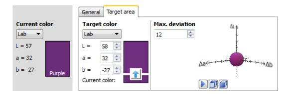
Current colour: The colour currently detected is displayed here. You can view the values for the colour currently detected in various colour spaces (RGB, Lab, LCh, HSV).
