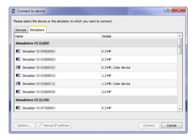
On the *Simulators* tab, you can connect with one of the simulators to simulate a device and modify job settings and device settings without having to connect to an actual device.
