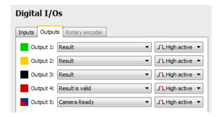
Enter how the outputs are to be activated here. Hardware signals (image trigger permitted, result valid, result, alarm, flash sync, device activated, heat warning, heat shutdown) can be issued for each output or the output configured for issuing job results.
