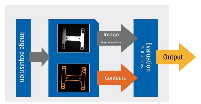
Here, each inspection task ("job") is divided into several feature checks. Each feature check executes one task and returns an associated pass/fail result or the associated measured values. For this purpose, a field of view must be defined that is either circular, an arc, rectangular or polygonal. The contours can be given via search arrows for geometrical feature checks.
