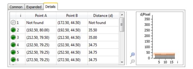
On the *Details* tab, there is a table showing the results for the individual search beams and a bar chart. This tab is only used to display the values. You can zoom into the bar chart with the magnifying glass.
