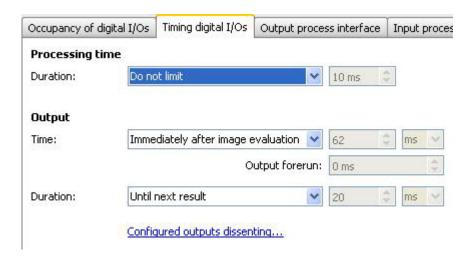
In this dialogue, you can define when the output time is reached and how long the output is to be. The timing diagram displays the process visually and you can mouse over various positions to bring up further details.
