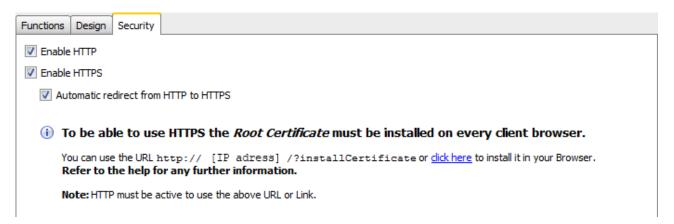
HTTP activation: Enable this function to transmit the data in unencrypted form.
