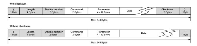
If you wish to transfer more than 65,535 bytes, e.g. jobs, you can extend the length to 8 bytes (sufficient for  $2^{32}$  bytes). This changes the start and end codes:
