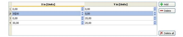
**4.** Enter the values for the marked coordinates. In this example, it is millimetres. Keep in mind that the coordinates must be specified with respect to a right-handed coordinate system (X towards the right, Y towards the top). The *Application Suite* suggests values for you, correct them if necessary.
