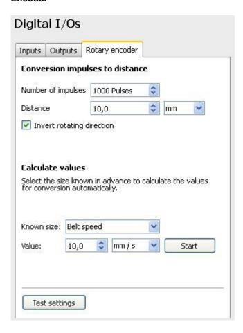
If an incremental encoder is connected, you must also set the factor between the distance travelled and the number of pulses from the encoder.
