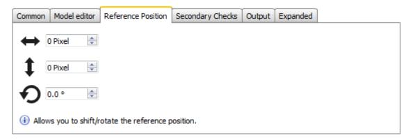
The reference position is by default the centre of the work area. The coordinates of this point can be output for each located object via the process interface.
