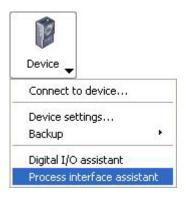
You can use the process interface assistant to check what data is being sent and received via the device process interface. It appears in chronological order in the *Device communication* field.
