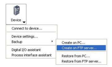
This dialogue page allows you to create a complete device backup of your device on the FTP. Here device settings, jobs and firmware are saved in a file.
