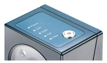
A screw and 5 LEDs are located on the Vision Sensor for displaying the various states.
