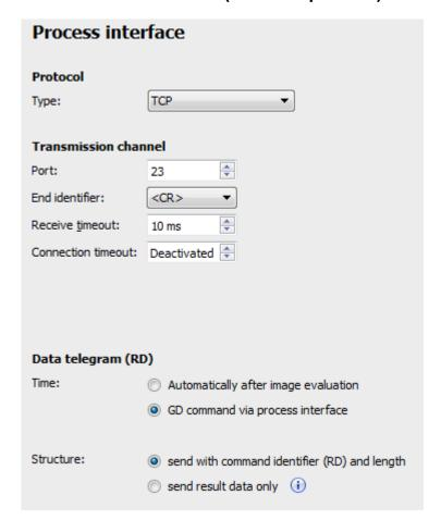
Here, you will find all parameters which can be used to configure data exchange via the interfaces.
