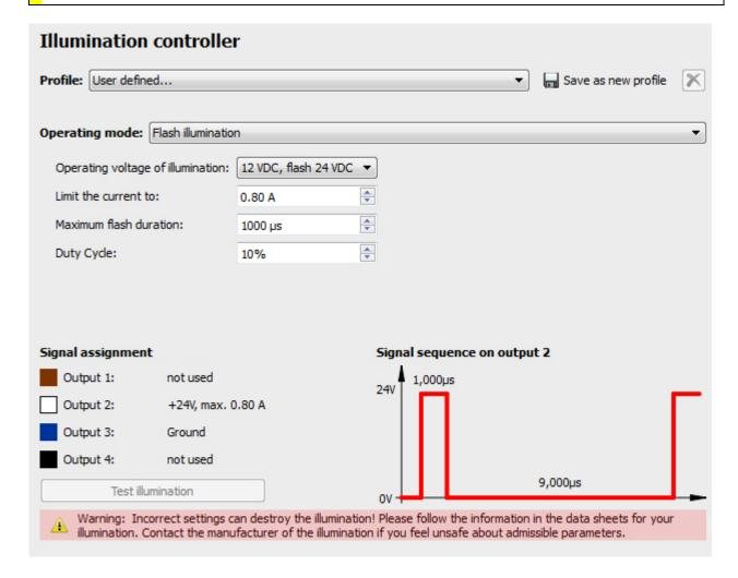
Using the illumination controller, you can make the settings at the outputs of the illumination port.
