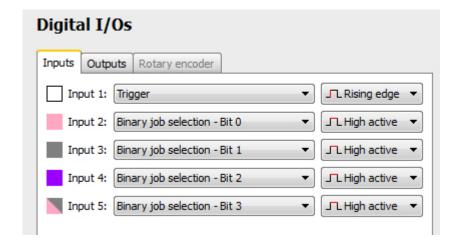
Input 1 is reserved for the trigger. For other inputs you can specify how you want to switch the active job. It is also possible to connect an incremental encoder to the Inputs 5 (CH-A) and 4 (CH-B).
