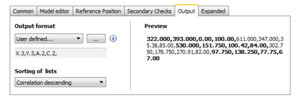
The *Output* tab can be used to define the content and structure of the *Formatted* list that can be output using the process interface. The *Formatted* list contains information about the located objects. The *Preview area* on the right displays the effect the settings have on the Formatted list in a live view.
