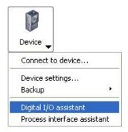
With the Digital I/Os assistant, you can test whether all cables are connected correctly to the digital inputs and outputs. To use the illumination controller, the device must be in Configuration mode.
