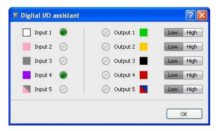
In the example, applied power is registered on Input 1 and Input 4.
