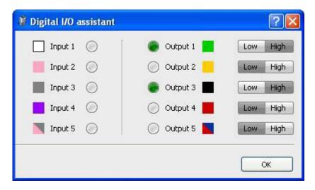
Set the appropriate output on or off using the Low/High button.
