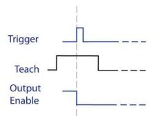
The digital input "Teach" must be in the "active high" state at the trigger point.
