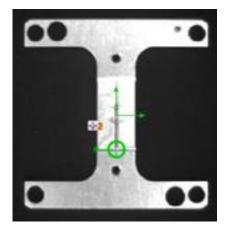
Set the point on the position to be determined. You may need to rotate it with the lever.
