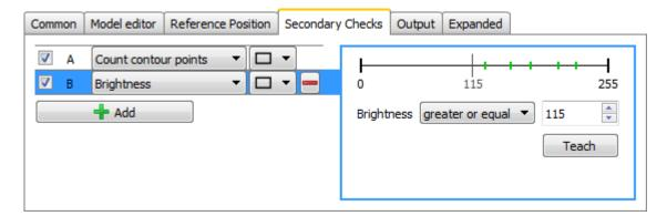
The *Additional tests* tab can be used to determine the criteria for subsequent testing of each located object. This enables detection of overlapping objects, for example, by stipulating criteria in their vicinity or on the surface of the object.
