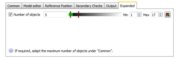
The *Extended* tab can be used to govern the result of the feature check regarding the number of located objects.
