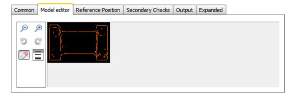
The Model editor tab can be used to edit the contours of the programmed object.
