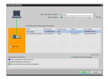
10. You have to open Non-grouped devices and use the TIA project to click on the Vision Sensor and Online & Diagnostics to assign a permanent IP address and a device name for the Vision Sensor.
