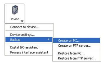
This dialogue page supports you in making a complete device backup of your device on the PC. Here device settings, jobs and firmware are saved in a file.
