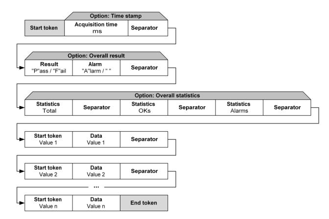
The time stamp in the datagram consists of 8 ASCII characters which specify the number of milliseconds since the system start of the device as a hexadecimal number. This value reverts from 4,294,967,295 ms to the value 0 ms after about 49.7 days.
