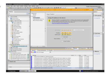
**11.** Click Assign PROFINET device name and assign a chosen name for the Vision Sensor.
