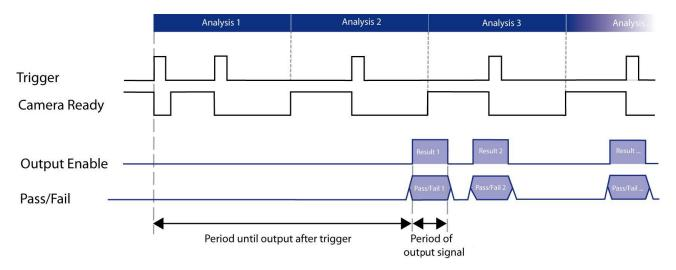
Following image acquisition, the *Image trigger permitted* signal is deactivated. The *Image trigger permitted* signal is activated again at the end of image acquisition and another image acquisition operation is possible immediately.
