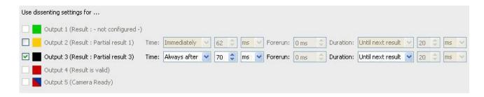
In this example, only output 3 has a different output time, although output 2 is also in use. They both follow the general output time.
