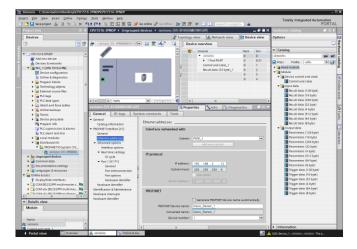
4. Configure the PROFINET cycle time (4 ms is advisable) in which data is to be transmitted.
