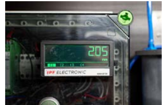
The pulse monitor currently contains four press-in dimensions (C1 to C4) for the negative matrices that can be selected at the touch of a button. The front panel unit visualizes the current dimension for the advance with green digits. The display changes to red when the target value for the depth of the die is reached. (Picture: ipf electronic)
