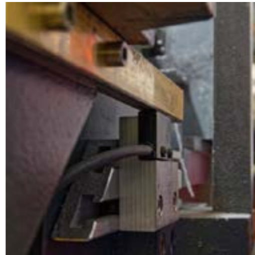
The sensor MW110430 is mounted on the machine so that the connection cable is not subject to wear. Above the sensor is the magnetic tape attached to the tunnel drive and protected from dirt by an additional stainless steel band. (Picture: ipf electronic)
