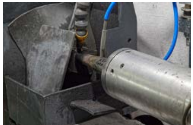
A negative matrix soldered onto an ultrasonic head is used to work the corresponding shape into the stone. The addition of boron carbide during the process is also clearly visible. (Picture: ipf electronic)
