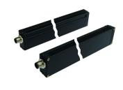
The multi-function light barriers are through-beam sensors where multiple beams are integrated. In case of interruption of only one beam, the switching output of the receiver changes its state. The devices are used where standard through-beam sensors with only one beam are not sufficient. There are devices with beam spacing of 20, 40, 60 or 120mm and different heights available. An integrated fuzzy logic controls the transmitting power automatically.
