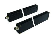
The multi-function light barriers are through-beam sensors where multiple beams are integrated. In case of interruption of only one beam, the switching output of the receiver changes its state. The devices are used where standard through-beam sensors with only one beam are not sufficient. There are devices with beam spacing of 20, 40, 60 or 120mm and different heights available. An integrated fuzzy logic controls the transmitting power automatically.
