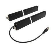
The multi-function light barriers are through-beam sensors where multiple beams are integrated. In case of interruption of only one beam, the switching output of the receiver changes its state. The devices are used where standard through-beam sensors with only one beam are not sufficient. There are devices with beam spacing of 20, 40, 60 or 120mm and different heights available. An integrated fuzzy logic controls the transmitting power automatically.
