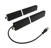
The multi-function light barriers are through-beam sensors where multiple beams are integrated. In case of interruption of only one beam, the switching output of the receiver changes its state. The devices are used where standard through-beam sensors with only one beam are not sufficient. There are devices with beam spacing of 20, 40, 60 or 120mm and different heights available. An integrated fuzzy logic controls the transmitting power automatically.
